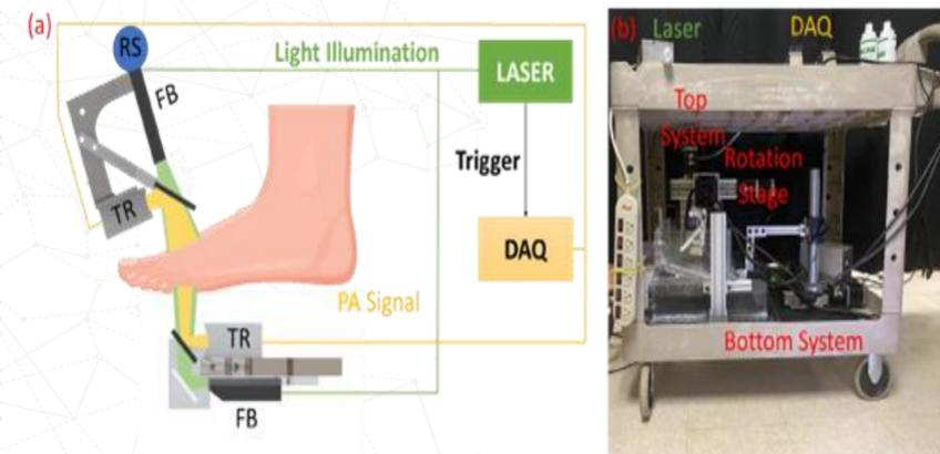
Figure 1. Experiment setups of the dual-scan imaging system. (a) A schematic drawing of the dual-scan PAT system. (b) A photograph of the system. All equipment is installed on a cart except the portable laser.
