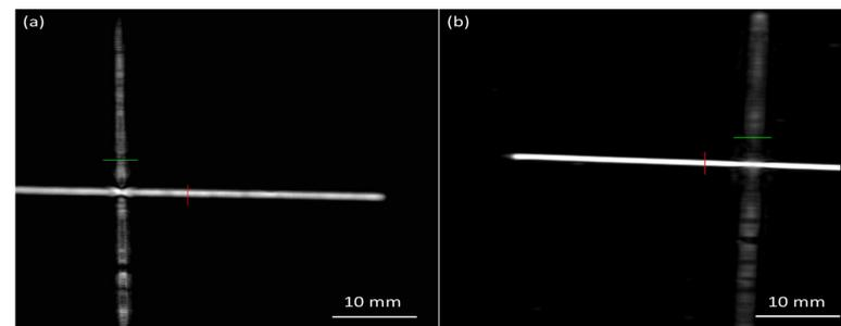
Figure 4. Spatial resolution quantification based on 0.2 mm width cross-line phantom
